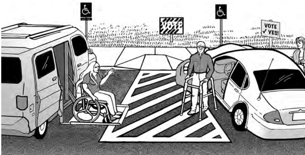
A van accessible parking space and a car parking space share an access aisle
